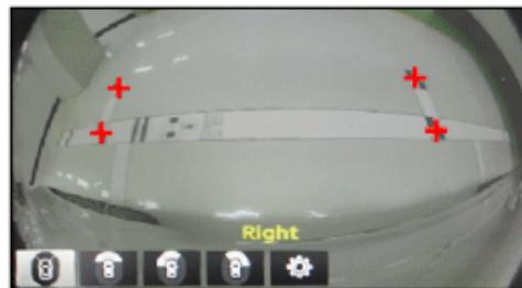
10. To confirm completion of calibration, check the vehicle and calibration line on AVN monitor and click [OK].
